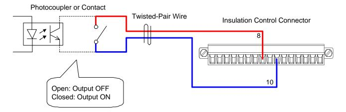
Toggling Output ON/OFF with Insulation External Contacts
