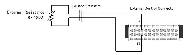
Output Voltage Control with External Resistance (B)
