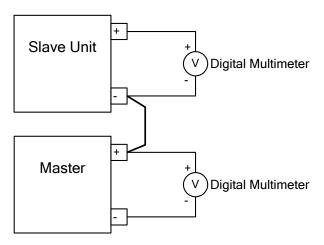
2. At the Master, set the constant voltage setting value to [xV] and the constant current setting value to [yA] and set the output to ON.
