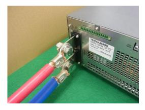
3. Put a insulation tube to the output cable and output terminal. And the insulation tube fix with Insulation lock.
