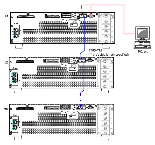
Controlling HX-G2 Series power supplies on multiple channels via computer
