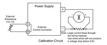
2. Set the constant voltage setting value to [ xV ] and the external resistance to infinity (open) and set the output to ON.
