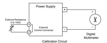
2. Set the external resistance to  $10k\Omega$  and the constant current setting value to [ yA ] and set the output to ON.
