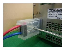
5. Attaching the output terminal cover is completed.
