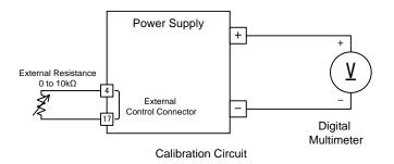
2. Set the external resistance to  $0\Omega$  and the constant current setting value to [ yA ] and set the output to ON.
