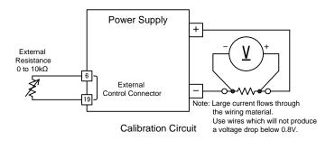
2. Set the constant voltage setting value to [ xV ] and the external resistance to  $0\Omega$  and set the output to ON.
