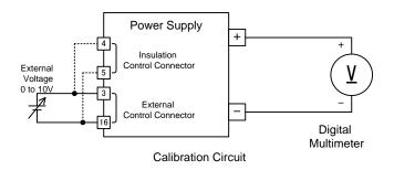
Set the external voltage to 0.010V and the constant current setting value to [ yA ] and set the output to ON.
