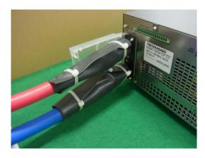
5. Fix the other output terminal cover on the right-side grooves of the output terminal.
