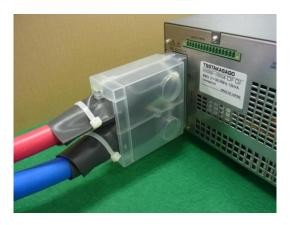
6. Fasten the output terminal covers with an M3X6mm screw. Attaching the output terminal cover is completed.
