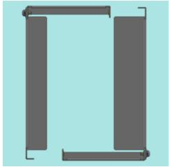
3. Snap the terminal covers together at the top and bottom along the groove on the terminal.
