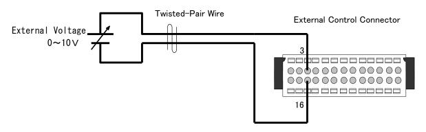
Output Voltage Control with External Voltage
