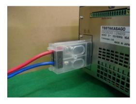
4. Fasten the output terminal covers with an M3X6mm screw.
