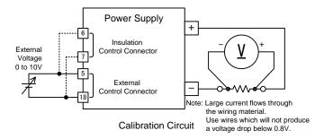
Set the external voltage to 0.010V and the constant voltage setting value to [xV] and set the output to ON.
