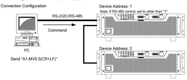
② Set voltage to 7.5V for HX-G2 power supply with device address set to 2.
