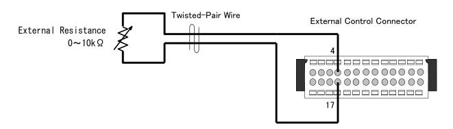
Output Voltage Control with External Resistance (C)
