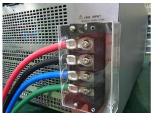
2. Tighten L1, L2, and L3 cable to the terminal block with screws.
