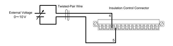
Output Voltage Control with Insulation External Voltage
