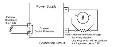
2. Set the constant voltage setting value to [ xV ] and the external resistance to  $10k\Omega$  and set the output to ON.
