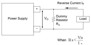
Reverse-Current Absorption by Dummy Resistor
