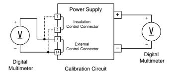
2. Set the parameter for FUNCTION item 12 to "0" to disable Linearity Compensation Function.
