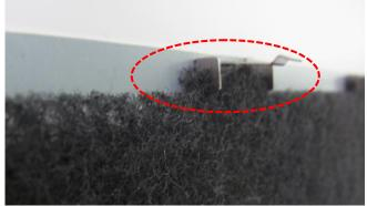
Air filter attachment is completed after inserting the filter into the lower hocks on the back-side of the front cover.
