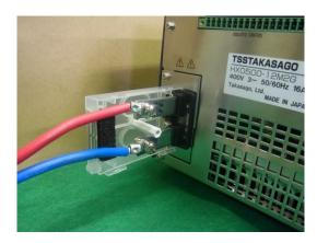
3. Fix the other output terminal cover on the right-side grooves of the output terminal.
