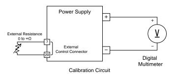
2. Set the external resistance to infinity (open) and the constant current setting value to [ yA ] and set the output to ON.
