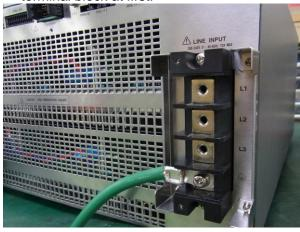
3. Mount the terminal cover to the terminal block with the appended M3 screw.
