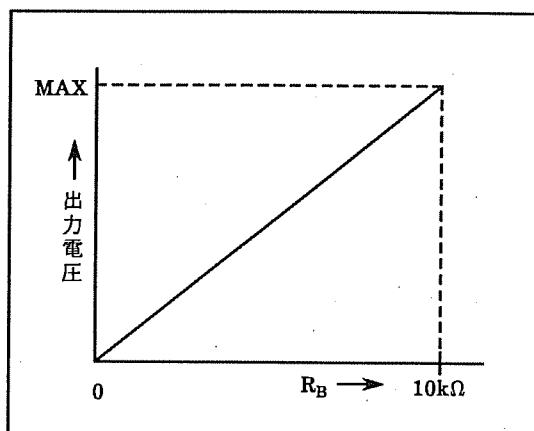
$$\text{出力電圧 (V)} = \frac{\text{最大出力電圧 (V)} \times \frac{R_B (\text{k}\Omega)}{10}}{10} \quad \text{----- (2)}$$
