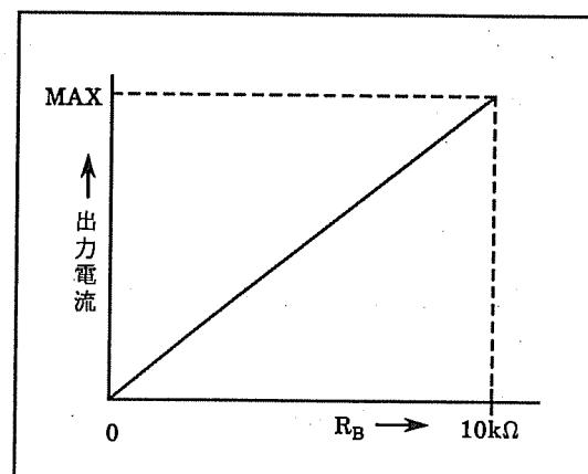
$$\text{出力電流 (A)} = \frac{\text{最大出力電流 (A)} \times \frac{R_B (\text{k}\Omega)}{10}}{10} \quad (5)$$
