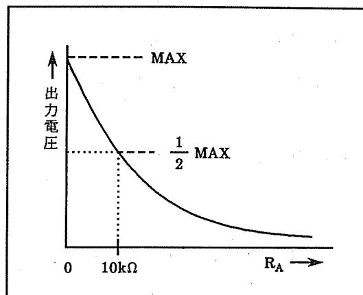
$$\text{出力電圧 (V)} = \frac{10}{R_A (\text{k}\Omega) + 10} \text{ (V)} \quad \text{----- (1)}$$
