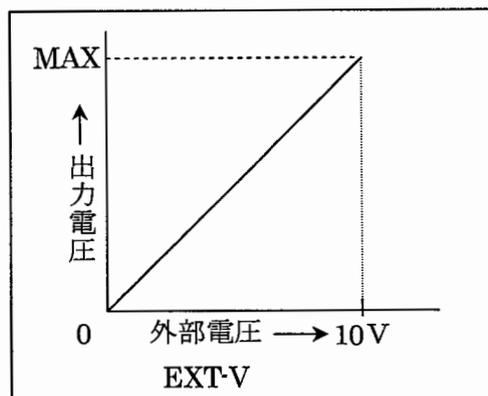
$$\text{出力電圧 (V)} = \text{最大出力電圧 (V)} \times \frac{\text{外部電圧 (V)}}{10} \quad (\text{V}) \dots\dots (3)$$
