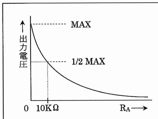
$$\text{出力電圧 (V)} = \text{最大出力電圧 (V)} \times \frac{10}{R_A(\text{k}\Omega) + 10} \quad (\text{V}) \dots\dots\dots (1)$$
