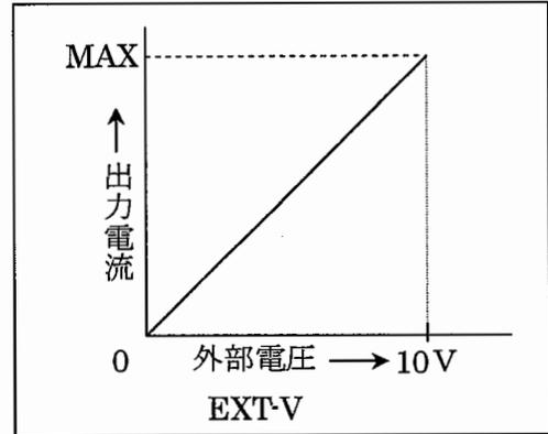
$$\text{出力電流 (A)} = \text{最大出力電流 (A)} \times \frac{\text{外部電圧 (V)}}{10} \quad (\text{A}) \dots\dots\dots (6)$$
