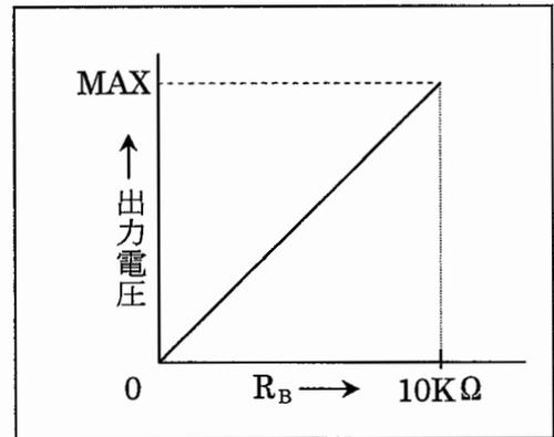
$$\text{出力電圧 (V)} = \text{最大出力電圧 (V)} \times \frac{R_B (\text{k}\Omega)}{10} \quad (\text{V}) \dots\dots\dots (2)$$
